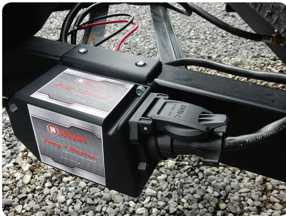
Hayes Towing Electronics' Sway Master is specially designed to eliminate annoying sway when weight distribution is not needed while also providing simultaneous braking to all brakes on a trailer when sway is detected. The plug-and-play device offers an easy install.
